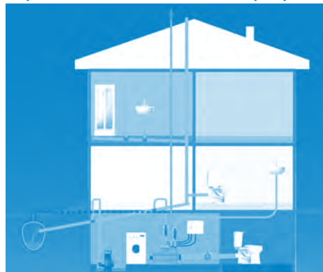
Figure 1: Example of installation with submersible pump:
